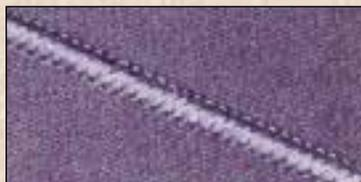
**2-THREAD FLATLOCK** uses one needle (left or right) and the lower looper thread *only*. This flatlock technique produces the flattest seaming when pulled taut.
