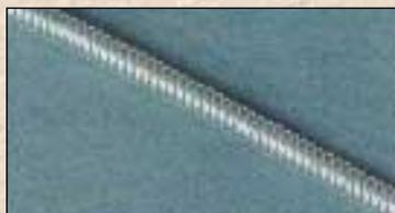
**3-THREAD FLATLOCK** uses a needle thread along with both the upper and lower looper. This stitch makes a strong seam, due to the needle and two loop-
