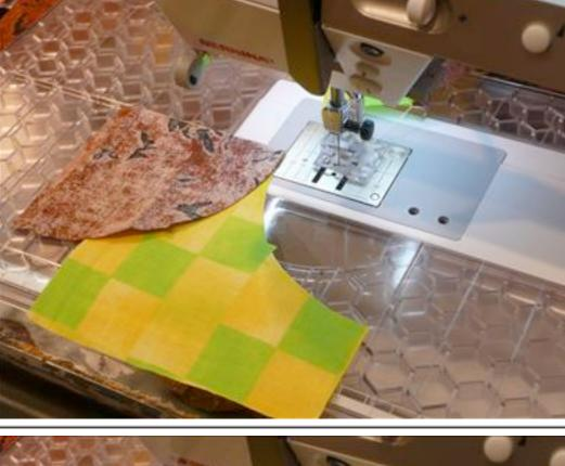
middle. No pinning at all. Note that the fabrics are placed together so that when you "flip them open"; they are aligned exactly as you want this edge of your block to appear.
