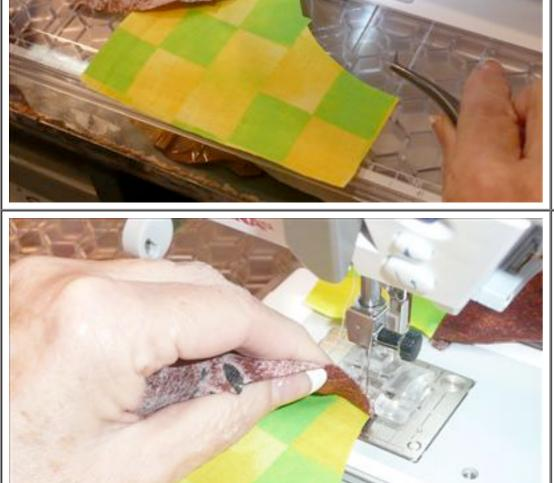
the top layer of fabric almost vertically, keeping your fingers in front of the needle, close to the front of the presser foot, not off to the left hand side. Note: The needle is not meant to align with the centre of the Curve Master Presser Foot. It is designed to be slightly off centre to allow a true scant 1/4" seam to be sewn.
